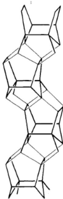
Figure 2: Chain building unit for ZSM-5 zeolite. 4
