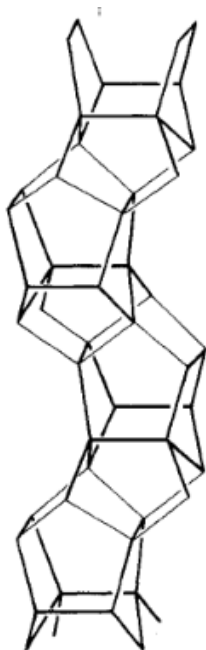
Figure 2: Chain building unit for ZSM-5 zeolite. 4
