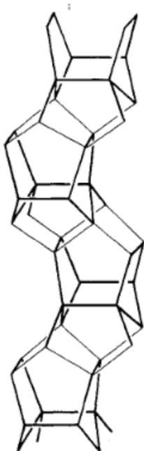
Figure 2: Chain building unit for ZSM-5 zeolite.<sup>4</sup>
