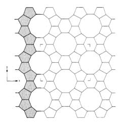
Figure 2: Chain building unit for ZSM-5 zeolite.  $^4$
